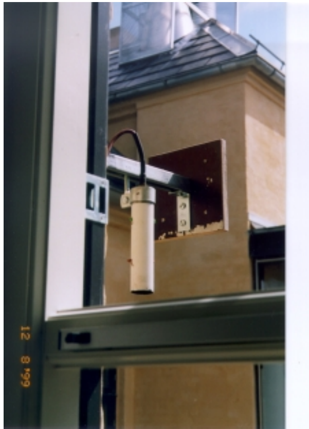
Figure 2.4. The shielded ambient temperature sensor and the back of the pyranometer.
