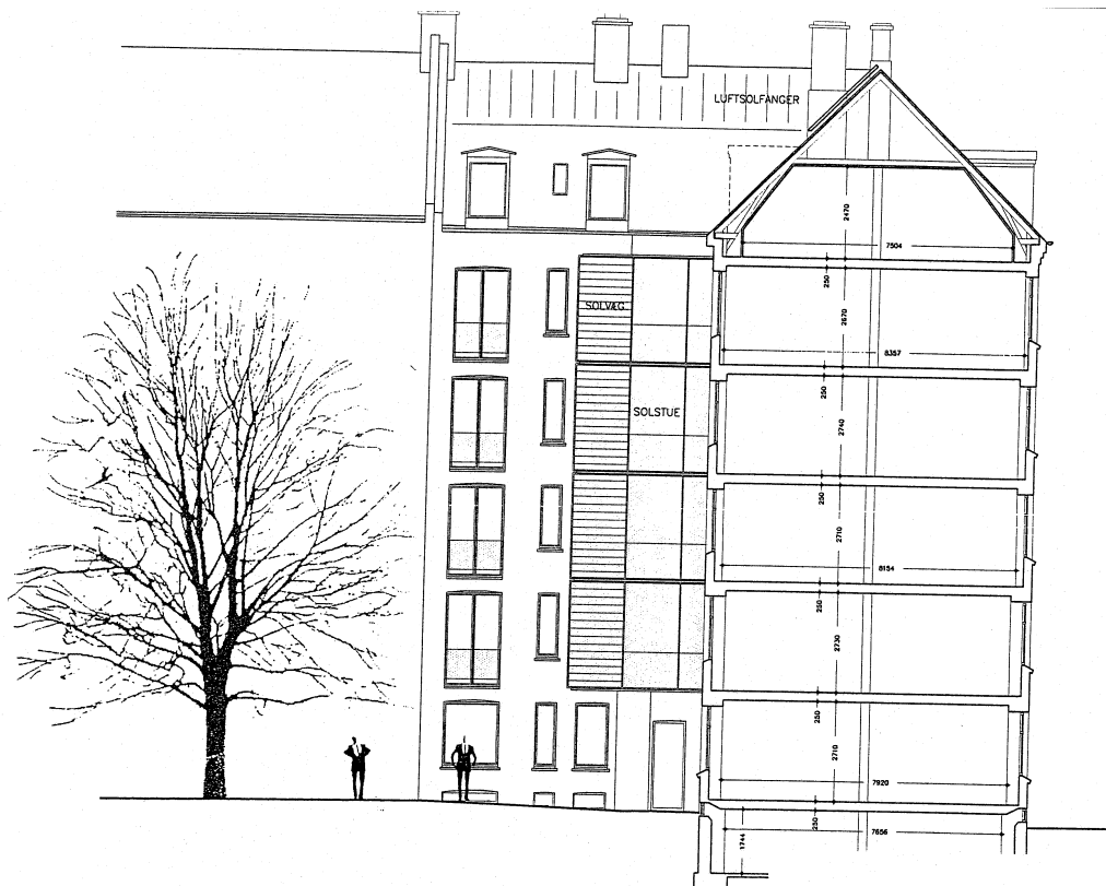
Figure 1.7. Drawing of the solar wall and sun spaces at Tøndergade 1.
