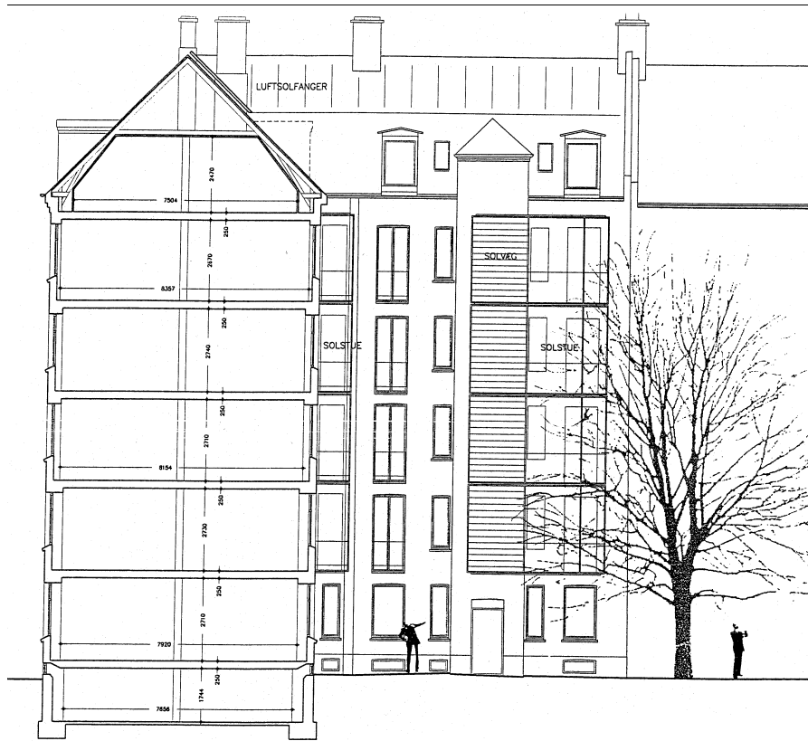
Figure 1.6. Drawing of the solar wall and sun spaces at Sundevedsgade 14.
