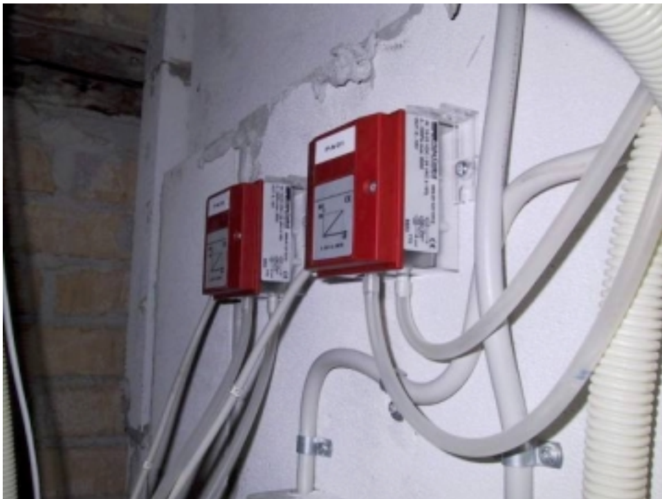
Figure 2.9. The pressure transducers for measuring the pressure drop across a calibrated orifice and a calibrated bending.
